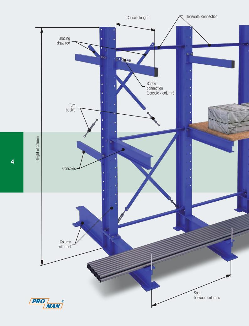
Cantilever racks are used mostly for the storage of long parts without the need to use pallets. Parts can be packed to bundles or stored individually. Racks are designed for indoor installation to storage halls and industrial buildings, as well as to the outside, but always on high-quality concrete floor.
