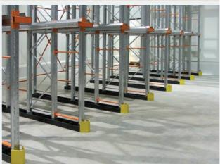
When designing the configuration of a drive-in rack, it is important to know the type of forklift used. It is possible to supplement the setup of the drive-in rack with racking accessories, e.g., forklift guides, upright protectors, pallet backstops for the far end of the lane, etc.
