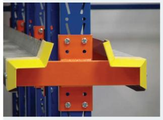
The steel rails are either single- or double-sided and are bolted to the upright frames using a bracket. Drive-in racks also contain a portal support beam located at the top of the upright frame for guaranteeing the frames' rigidity. There are vertical and horizontal bracing rods to ensure the stability of the drive-in rack.
